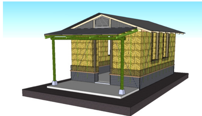
The Ti Kay Pay unplastered, showing mesh over gravel bags, bamboo stiffeners over straw bales, and diagonal wire bracing
